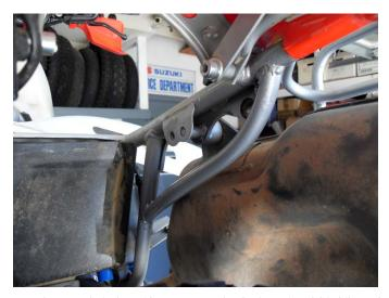
As you may have read in a earlier post, we discovered a couple of minor things to adjust and change on Larry's Honda XR650L after it's break-in ride. We also wanted to add some reinforcement to the bike's sub-frame. While the Honda is a stout machine, as evidenced by several Baja 1000 wins, when you load up a bunch of stuff on aftermarket racks you will tax the stock sub-frame.
